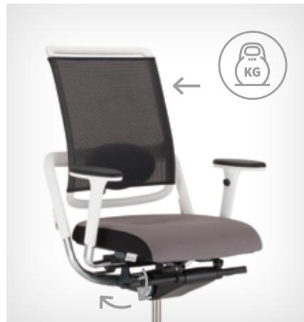
Backrest resistance force can be adjusted from 45 to 110kg with an easily-accessible crank. A range of backrest tilt force adjustment for users weighing from 85 to 150kg is also available.
